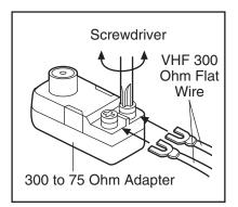
2. Push the 300 ohm to 75 ohm adapter onto the 75 ohm antenna terminal on the treadmill frame near the power cord.
